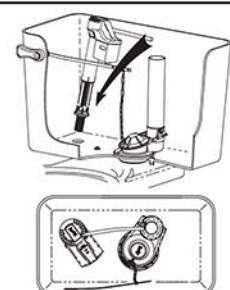
Place locked valve in tank so refill tube has direct path to flush valve.
