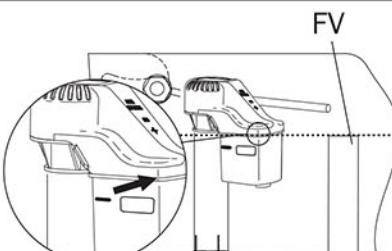
Press down until corner of white cover and top of flush valve (FV) line up. Note: If tower style flush valve (TS), match fill valve water line to water line marked in tank (stain line).
