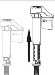
Turn top of new valve counterclockwise to unlock and pull up to fully extend.
