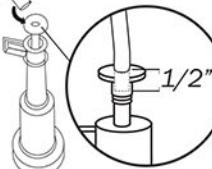
**Attach to overflow tube with metal clip.**
